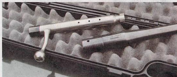
The large 3-lug bolt locks directly into the barrel, which is wrapped in a steel receiver; no complaints on strength here!
