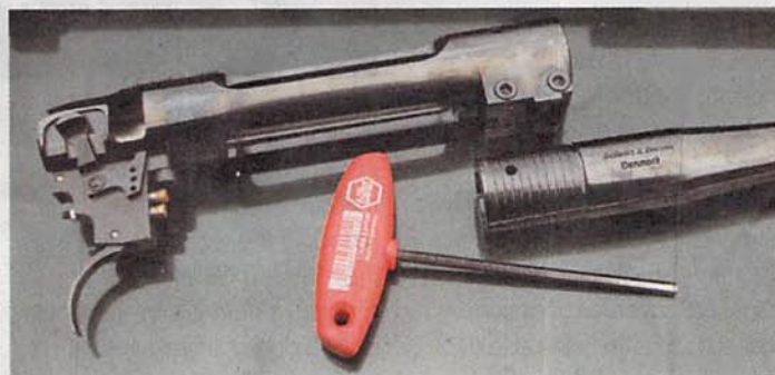
Barrel removed showing pinch retention system, the T-key is included, note the trigger adjuster screws for weight and length
