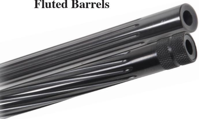
Available with a choice of straight or spiral fluting. Fluting reduces the weight of the barrel without reducing the stiffness of the barrel. Additionally, fluting provides a greater surface area for heat dissipation and because the bottom of the flute channel is closer to the bore, the heat reaches the surface more quickly further aiding cooling. Not all calibres are available from stock but may be to order.
